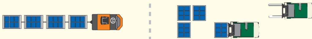
By towing loaded dollies linked in series, the CBT/CBTY can transport large loads at one time. A forklift must travel back and forth many times to transport the same load volume.
