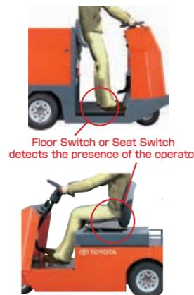
Floor Switch or Seat Switch detects the presence of the operator.
