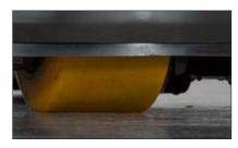
RUBBER BUMPER SKIRT Rubber skirting directs light debris away from the drive tire.
