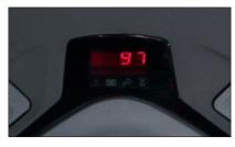
BATTERY DISCHARGE INDICATOR (BDI) WITH LIFT INTERRUPT
